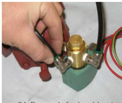
Figure 34: Removal of solenoid water supply lines
