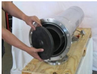
Figure 12: Removal of coarse screen cap
