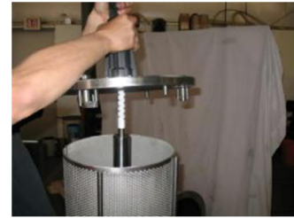
Figure 22: Upper bulkhead removal
