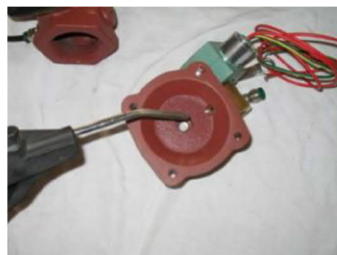
Figure 42: Removing water from cover plate
