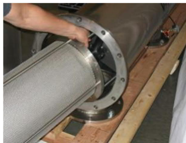
Figure 18: Supporting the internal assembly
