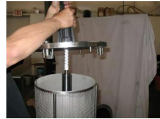
Figure 22: Upper bulkhead removal
