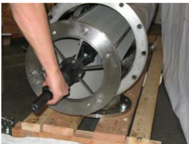
Figure 17: Internal assembly removal
