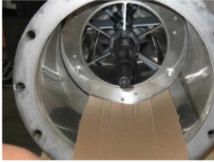
Figure 14: Covering the inlet line
