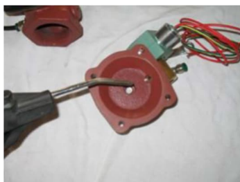
Figure 50: Removing water from cover plate.
