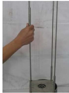
Figure 34: Removing lower sleeves
