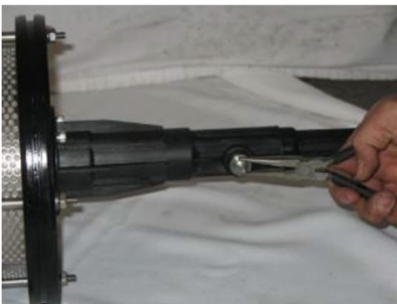
Figure 23: Removal of pawl
