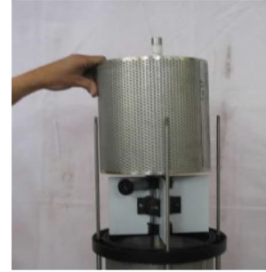
Figure 28: Upper screen removal
