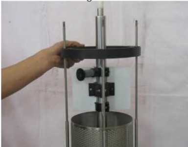
Figure 29: Removal center bulkhead
