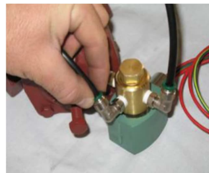
Figure 42: Removal of solenoid water supply lines
