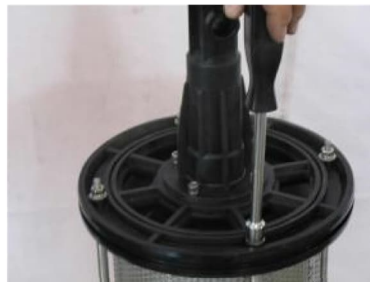
Figure 24: Removal of bulkhead nuts
