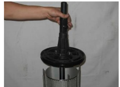
Figure 25: Removal of upper bulkhead
