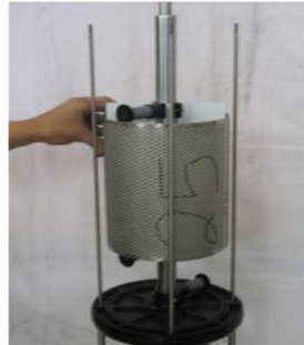
Figure 30: Removal of lower screen
