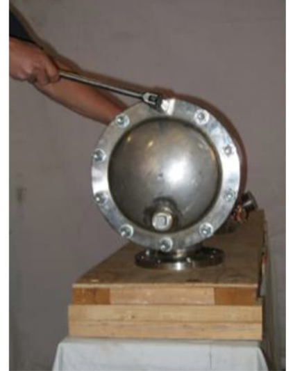
Figure 10: Removal of lid
