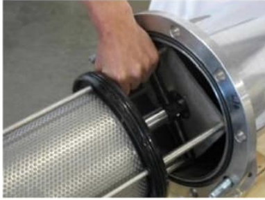
Figure 20: Supporting the internal assembly.
