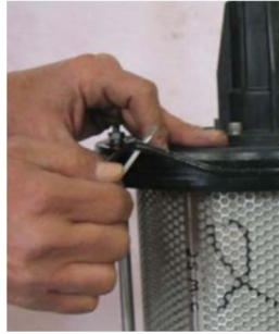
Figure 21: Removal of bulkhead seals
