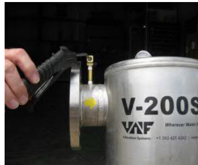
Figure 20: Blowing out air lines
