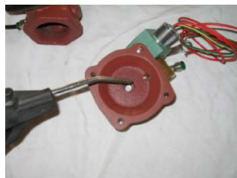
Figure 30: Removing water from cover plate
