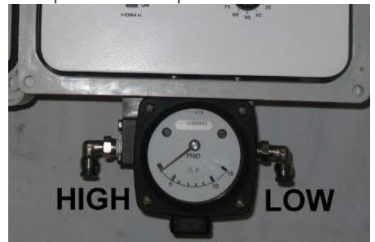
Figure 3: High & low-pressure ports on the DP switch/gauge
