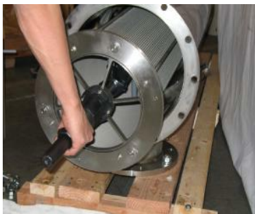
Figure 17: Internal assembly removal
