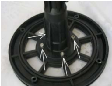
Figure 23: Reverser housing mounting screws
