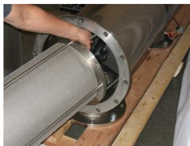
Figure 18: Supporting the internal assembly
