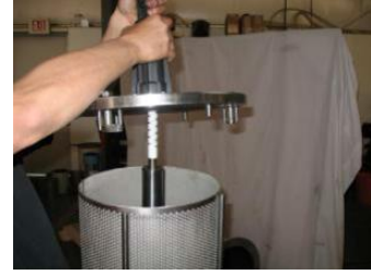
Figure 22: Upper bulkhead removal
