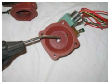
Figure 42: Removing water from cover plate
