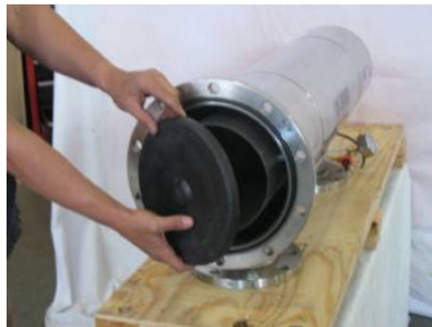
Figure 12: Removal of coarse screen cap
