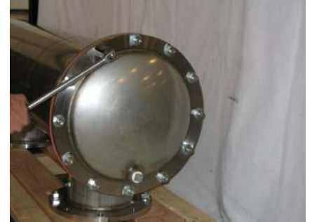
Figure 10: Removal of lid
