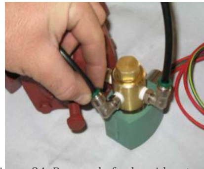
Figure 34: Removal of solenoid water supply lines
