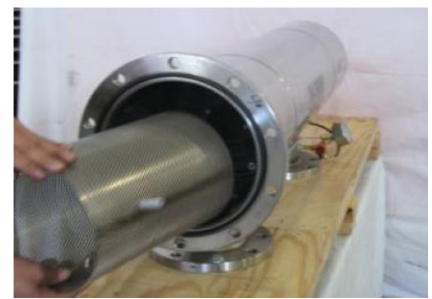
Figure 13: Removal of coarse screen
