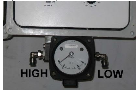
Figure 3: High & low-pressure ports on the DP switch/gauge
