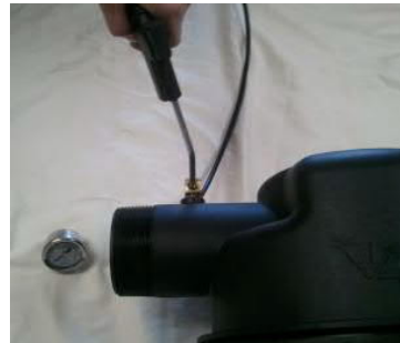
Figure 19: Blowing out air lines
