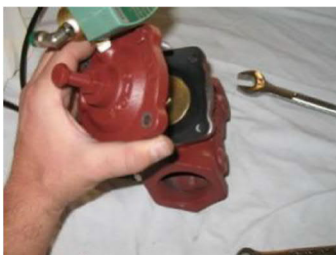
Figure 28: Removal of diaphragm cover plate
