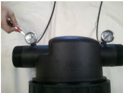
Figure 18: Removal of pressure gauge
