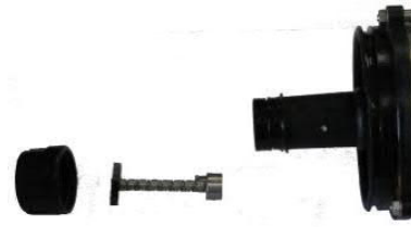
Figure 13: Removal of pawl removal
